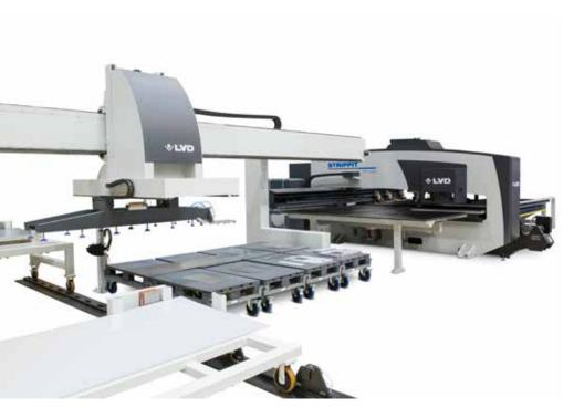
Flexible Automation (FA-P) offers advanced load/unload, part picking and a large area for stacking punched parts directly onto the allocated pallet.
